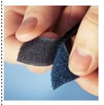
Velcro was invented by an engineer who got the idea from removing burrs from his dog's hair. Velcro uses strips or patches of a hooked material opposite strips
