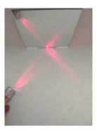
7. On the bottom of the box, use a pencil to mark the point where the laser hits the mirror and mark "N" for normal. Trace a small line along the laser ray and mark it "I" for ray of incidence. Trace a small line on the reflected laser ray and mark "R" for ray of reflection.
